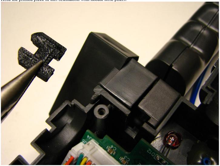
The curved edges are to the left and the shortest leg goes on the top right-hand side. This is because there is only a small lip in the inside handle piece so not much room to grab onto that piece.
