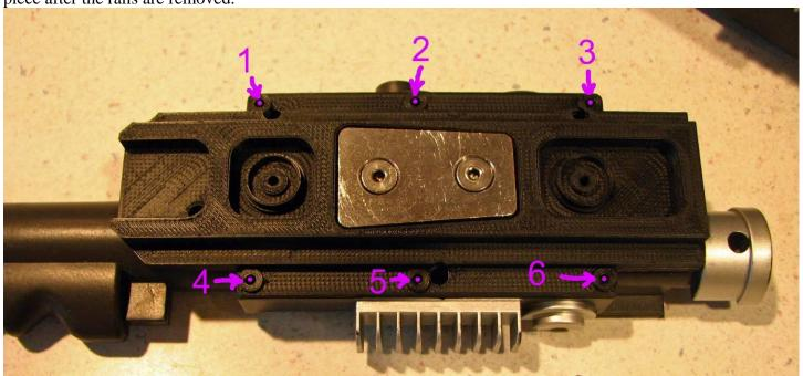
Remove the rails and then drill out the 6 holes with the slightly larger 3/32" drill bit at the 6 locations:
