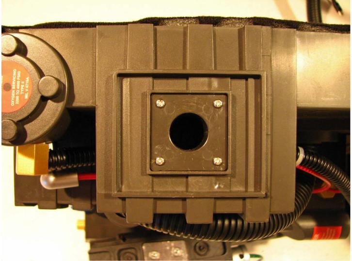
There are two different ways to mount the magnet, depending on whether the existing hole cover is used or not.
