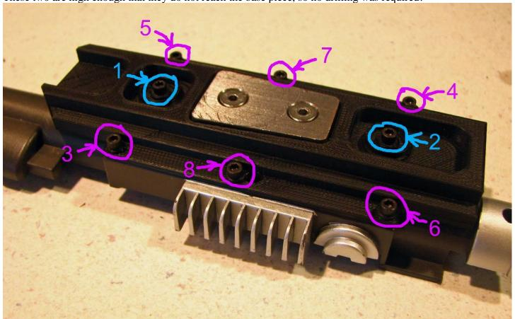
Then install the remaining 6 screws around the edges (#3-#8) in the suggested order shown in the above image.
