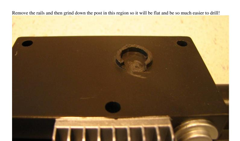
Now we need to drill the main two holes that will hold the rails and steel plate onto this Spirit Wand Bottom Piece. Place the rail on the bottom and align the rails so that it is centered on the bottom plate and tape it in place. There is some wiggle room to help aid in alignment in case of some variations in manufacturing the wand.
