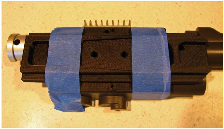
Now using the 1/8" bit, carefully drill down the center of the two holes where the steel plate will be mounted. The drill bit is smaller than the holes since we do not want to remove any material from the 3D printed rails and only want to mark the center of the holes in the bottom piece.
