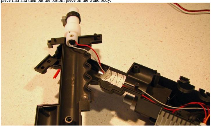
Now flip it over and press the two pieces together. At the back side, do not forget to make sure the green (or blue) tubing is in place before putting the screws back in. Find those 6 screws that you originally removed and put them back in. See the recommended order of installing the screws in the following image:
