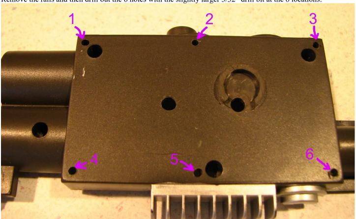
Now you get to reattach the steel plate and railing for possibly the last time! Align the steel plate and rails and slightly tighten it down to the base plate. Allow some ability to align the rails since we will be adding 6 screws that will also need to be able to get into their holes in the base piece.
