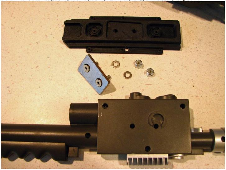
Using the 3/32" Hex Key and 11/32" socket, attach the steel plate to the rails and the Spirit Wand Base Piece and make sure the rails are well aligned before tightening.
