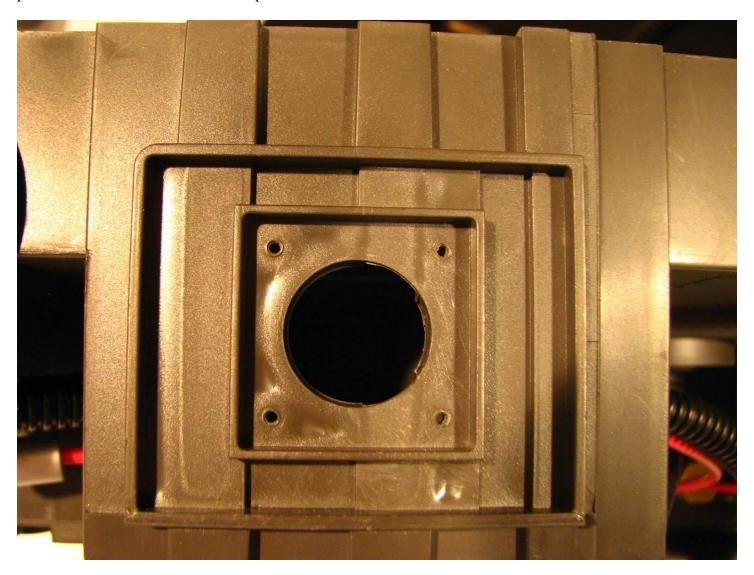
Place the shorter screw (part #7) through the magnet and the magnet on top of the hole shown above. It fits very nicely and is secured by the four raised walls that surround the hole. Without the molded plastic plate, the shorter screw reaches the inside of the pack and the fender washer (part #9) and lock nut (part #10) can be tightened down to hold the magnet in place.
