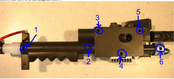
When lifting off the bottom plate, take care near screw #1. This can be a tight connection between the bottom piece and the white wand tip piece. Carefully pry the parts away from each other. There are also two wires that go around this post so do not damage those wires.
